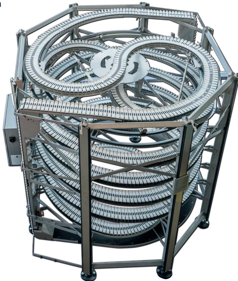
The AccuVeyor AVh has been designed to eliminate the limitations of traditional spiral accumulators. As a dynamic accumulator, it disconnects the successive processes/machines in packaging lines, filling lines, etc.
