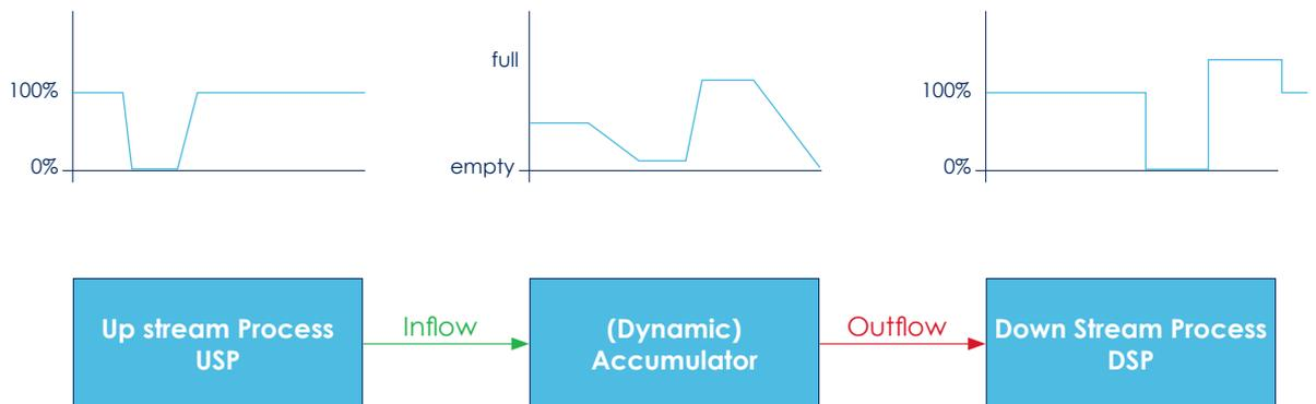
*Typical characteristics of discontinues processes balanced out by a Dynamic Accumulator.*
